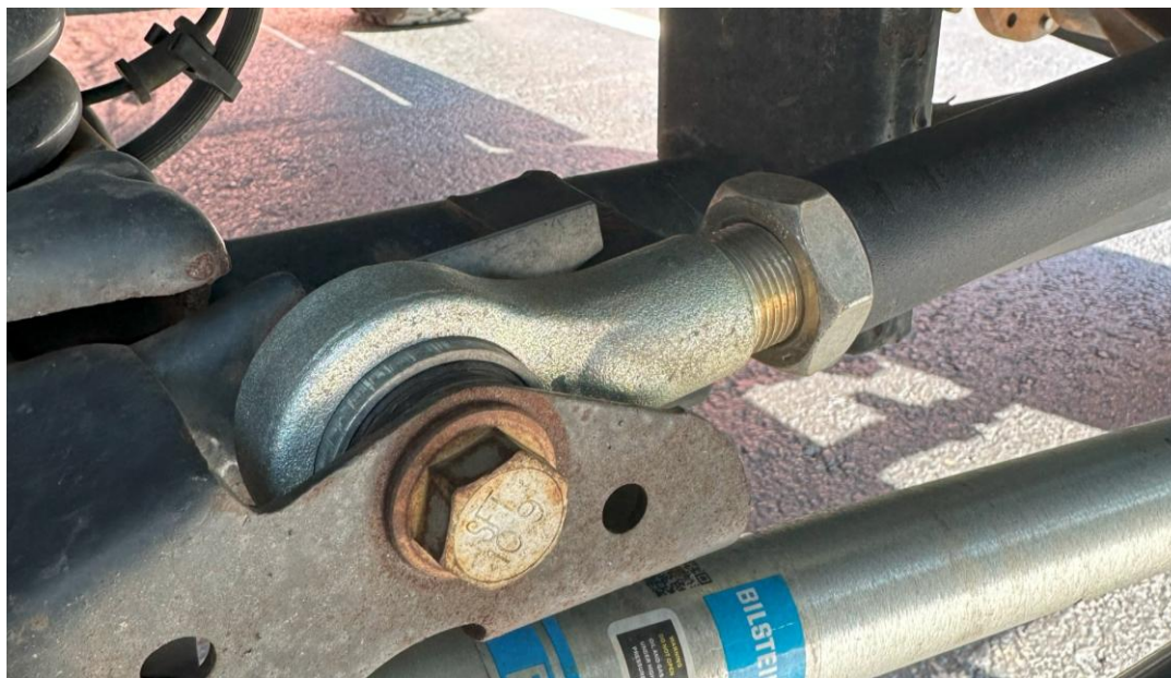
JK adjustable front track bar bolt installed hand-tight (axle-end)
