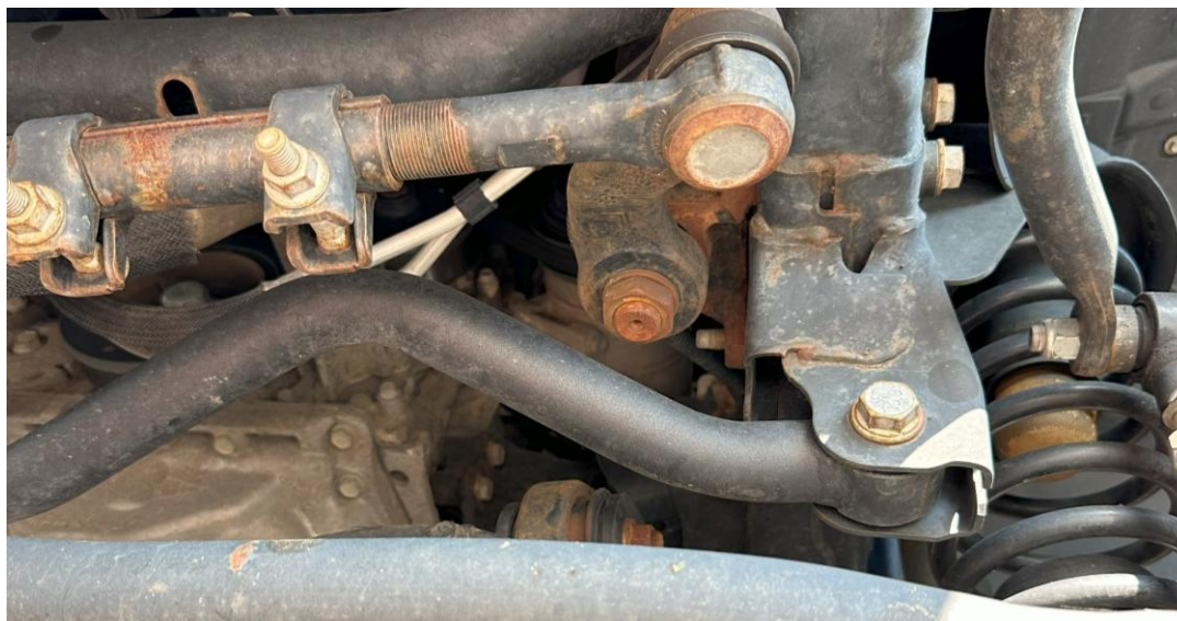
JK adjustable front track bar bolt installed hand-tight (frame-end)
