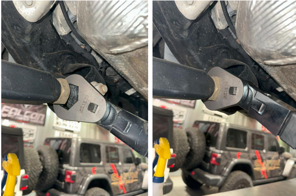
Figure 2: Crow's Foot Wrench slipped over threaded shank and onto jam nut
