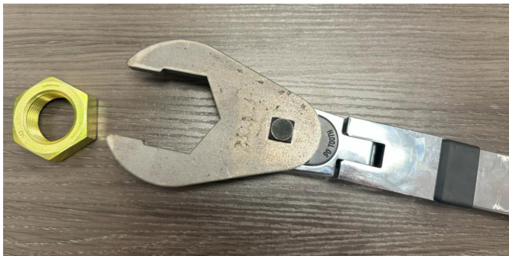
Figure 1: Torque wrench with new Crow's Foot Wrench
