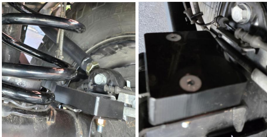
Figure 1: Extension located on bump stop perch with bolts dropped in holes
