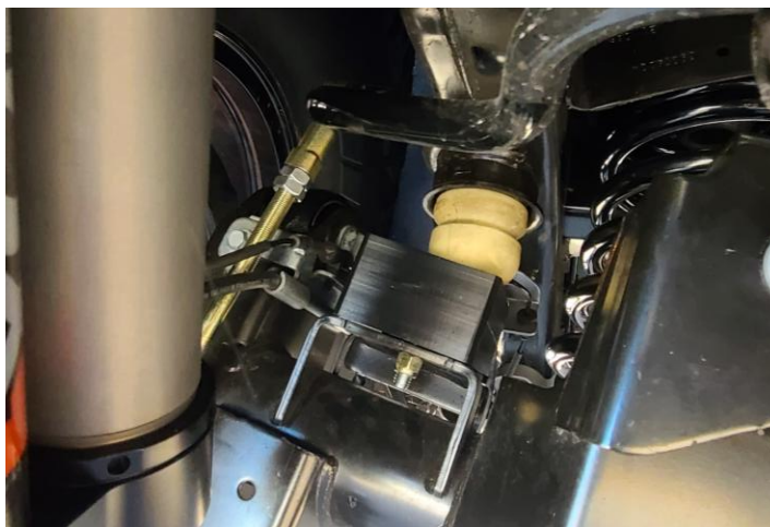
Figure 3: Installation photo (2x, 1" of bump stop used)
