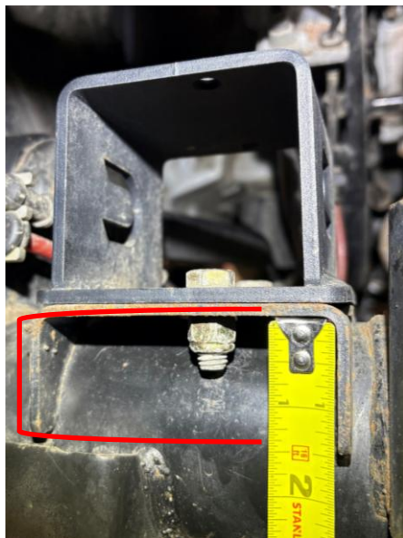
Short Bump Stop Pad on "Standard" JL's
