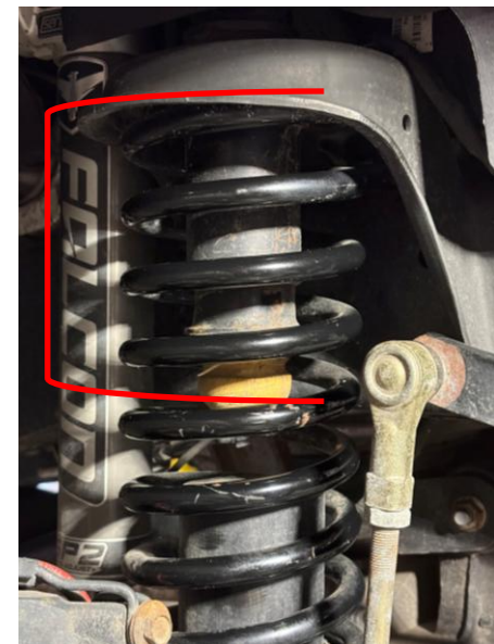
Short Bump Stop Tower on "Standard" JL's
